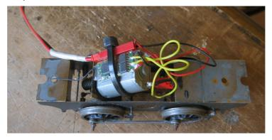
Once installed, the engine is switched on and off by connecting and disconnecting the JST leads which can conveniently be stowed in the cab or the coal bunker while running.
